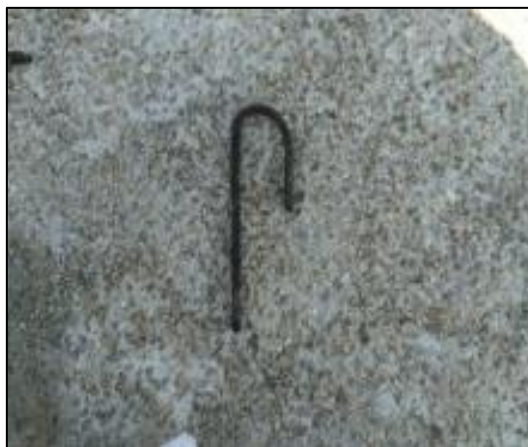
Figure 5. Plot retaining iron anchor (Permatasari et al., 2017)
